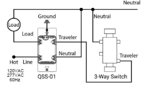
**Note:** For 3-way configurations, ensure the smart dimmer is installed in the junction box where Line (Hot) enters the electrical circuit. Insert wires into holes, do not wrap wires around screws. Do not remove screws. The Qoralux Smart Switch is designed to operate in either 120VAC or 277VAC circuits. For 277VAC 3-way circuits, use standard "off-the-shelf" 277VAC compatible 3-way switch.
