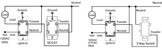
Note: For 3-way configurations, ensure the smart dimmer is installed in the junction box where Line (Hot) enters the electrical circuit. Insert wires into holes, do not wrap wires around screws. Do not remove screws.
