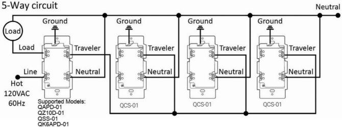
**Note:** For 3-way configurations, ensure the smart switch is installed in the junction box where Line (Hot) enters the electrical circuit. Insert wires into holes, do not wrap wires around screws. Do not remove screws.
