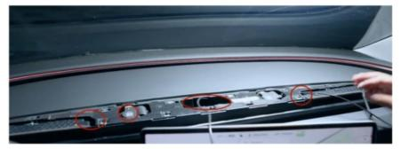
19. Run the wire through the instrument position above the front steering wheel
