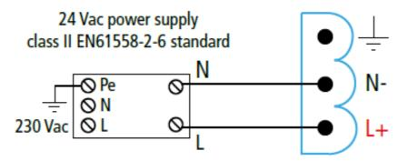
• For transmitters with 100-240 Vac power supply:
