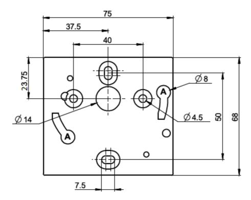
To mount the transmitter, mount the ABS plate on the wall (drilling: 50 Ø 6 mm, screws and pins are supplied). Insert the transmitter on the fixing plate (see A on the drawing beside). Rotate the housing in a clockwise direction until you hear a "click" which confirms that the transmitter is correctly installed.
