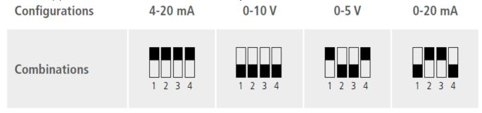
• Connection of the output in current 4-20 mA:
