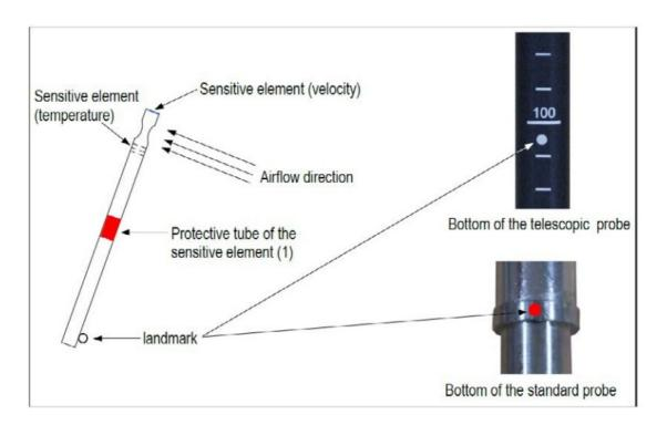
Before any use of the device with an air velocity probe, please lower the protective tube (1) of the sensitive element (except vane probe). Always use the standard air velocity probe with the red point in front of the flow. Always use the telescopic probe with the white point in front of the flow.
