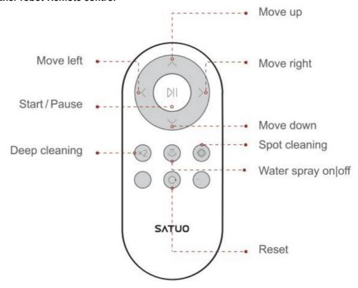
Rating: 3VDC AAA TYPE) Wireless Frequency: 433.92MHz
