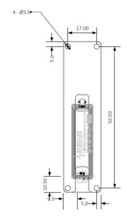
Dimensions of 090-10-005-ASY Ver: A 6-Turn Antenna (mm) (Equivalent for unit in SATO CL4XX and CL4NX Printer).
