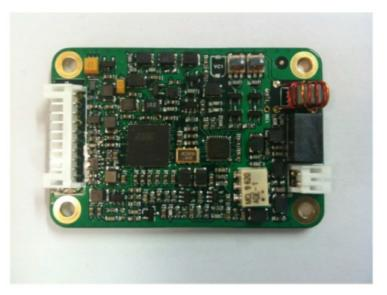
2. MR-1 Module Rev B1 with Shielding Can
