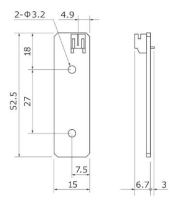
Dimensions of 090-10-010-ASY Ver: A 6-Turn Antenna (mm) (Equivalent for unit in SATO CG208 Printer).
