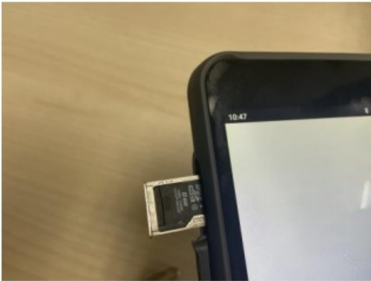
Figure 1-4-7 Installation of Micro SD card
