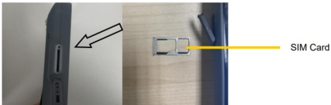
Figure 1-4-3 Installation of SIM card
