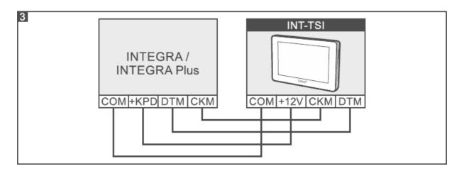
10. Connect the power wires to the +12V and COM terminals. The keypad can be powered from the control panel (Fig. 3), from an expander with power supply or from an additional power supply unit.
