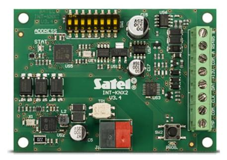
INT-KNX-2 is an expander module that integrates the functionalities of the advanced INTEGRA and INTEGRA Plus intruder alarm systems with the KNX building automation systems. This allows the two systems to communicate, with the KNX devices reporting their status directly to the alarm control panel which in turn can control these devices.
