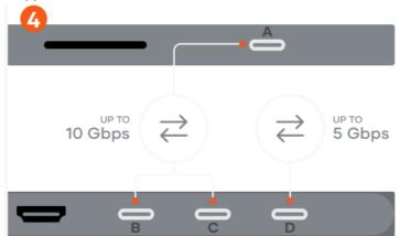
USB-C data ports allow for transfer data at up to 10 Gbps (A, B, C) and 5 Gbps (D) speeds. Does not support video output, charging or CD readers including the Apple SuperDrive.
