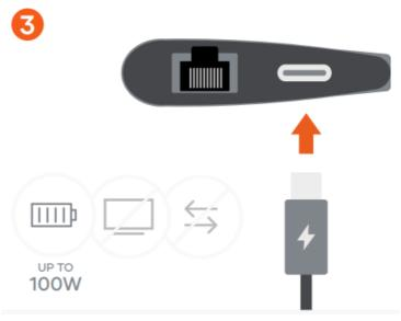
Use the USB-C PD port to charge your device up to 100W. ~15W is used for adapter operation. Video and data transfer not supported.
