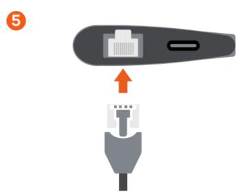
Connect an Ethernet cable to the adapter's Gigabit Ethernet port.
