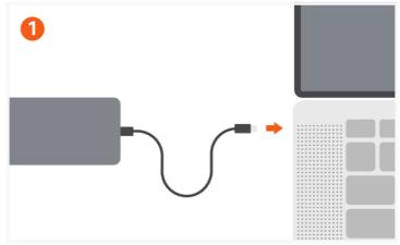
Connect the adapter to a compatible USB-C port on your host device.
