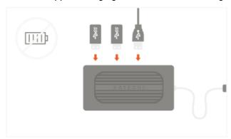
5. Connect an RJ45 network cable to the adapter's Gigabit Ethernet port.
