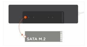
3. Insert the SSD (not included) faceup with the pins aligned and push down on the screw to secure it into place. Supports SATA M.2 SSD only, does not work with Nvme
