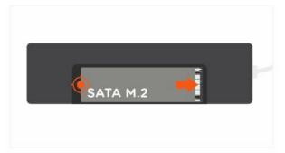
4. Once the SSD is secured, slide the cover back onto the adapter.
