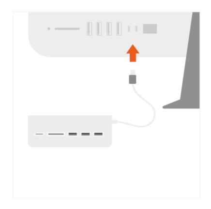
Use the USB-A data ports to connect three USB devices or peripherals.
