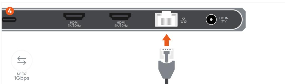
Connect an RJ45 Ethernet cable to the Dock's Gigabit Ethernet port. Up to 1Gbps
