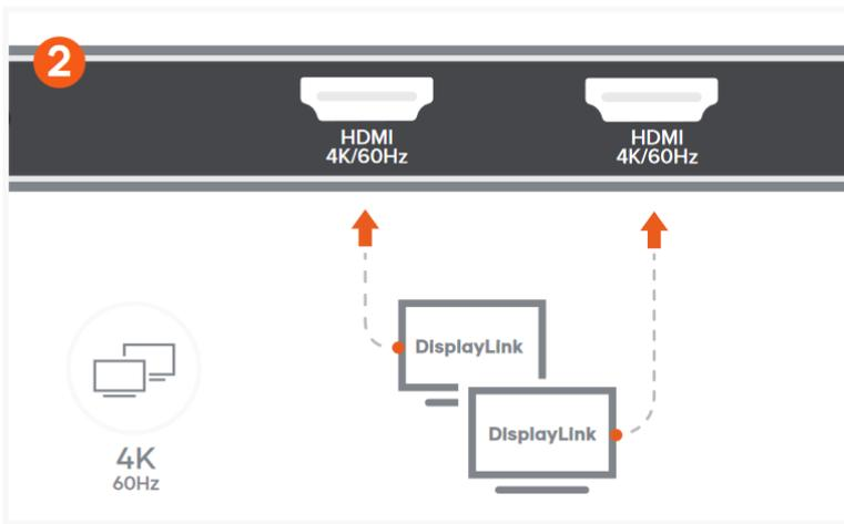
Use HDMI ports to connect up to two HDMI-enabled monitors. Supports 4K/60Hz each. DisplayLink Manager must be installed to use HDMI ports.
