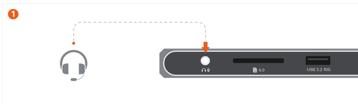
Attach audio device to the 3.5mm Audio I/O jack.
