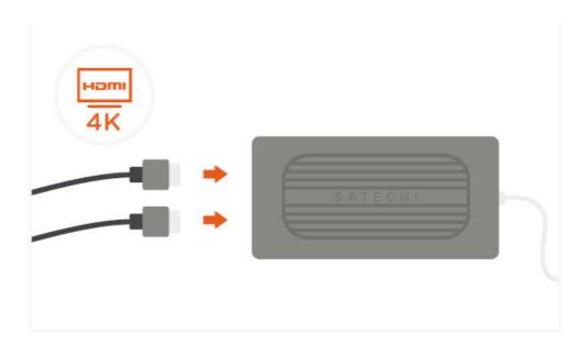
Use the USB-C PD charging port to power your device – up to  $100W \sim 15W$  of power used for operation USB-C charging port does not support video or data
