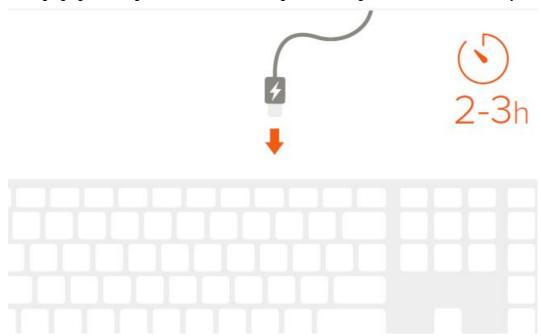
5. The keyboard can be used in wired mode by pressing "Fn + Eject" while the cable is connected. Press "Fn + Bluetooth key" to switch back to wireless mode
