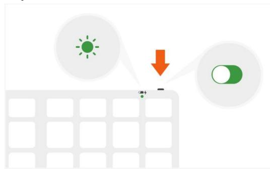
2. Press and hold one of the keyboard's Bluetooth keys for ~3 seconds, until the LED light starts to blink. Select "Slim X3 Keyboard" on the host device's Bluetooth settings to complete the pairing process. Repeat for each button to connect up to four devices
