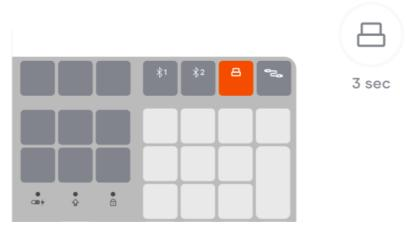
6. To use the keyboard in wired mode connect the included cable, press and hold the wired mode key to switch the keyboard into wired mode connection.
