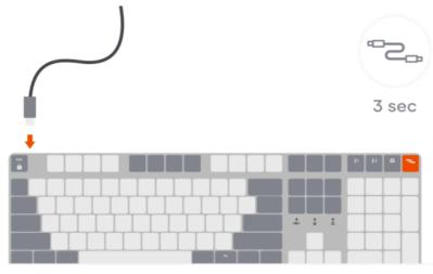
7. To recharge, connect the included USB-C power cable to the USB-C port on the keyboard, the charging LED will illuminate.
