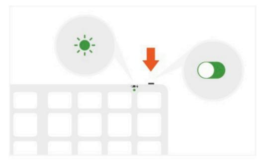
2. Press and hold one of the keyboard's Bluetooth keys for 3 seconds, until the LED light starts to blink. Select "Slim X3 Keyboard" on the host device's Bluetooth settings to complete the pairing process. Repeat for each button to connect up to four devices
