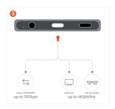
Connect a Thunderbolt 4, USB4, or USB-C to HDMI/DP cable to the USB-C port. Supports USB 3.0 at 10 Gbps, 2-lane DP1.4 with 8.1 Gbps per lane, 4-lane DP1.2 for iPhone 15, 4K@60Hz mode depending on the host and screen.
