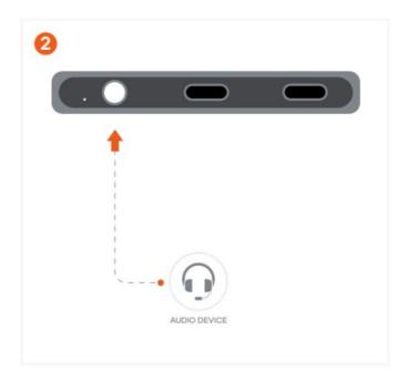
Insert an audio device into the 3.5mm auxiliary port.
