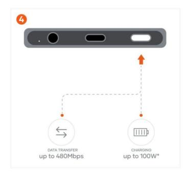
Connect a USB-C charging cable to either USB-C PD port. Supports USB 2.0, plug & play; PD3.1 SPR, with a maximum input up to 100W depending on the host device.
