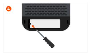
Secure the SSD using the included screwdriver and screw. **Tip:** To prevent stripping the screw, do not overtighten
