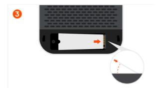
Insert the SSD at a slight angle (35-45°) and ensure it is fully seated in the PCIe slot.
