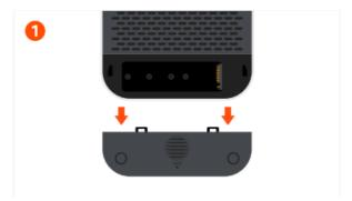
Remove the SSD enclosure cover on the bottom of the stand.
