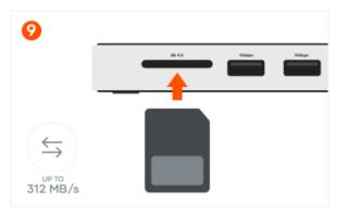
SD 4.0 Card Reader (up to 312 MB/s) High-speed data transfer for SD cards. Insert the card with the label facing up and the pins facing down.
