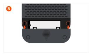
Carefully reattach the enclosure cover: insert the side clips first, then slide the door into place.
