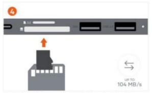
Insert micro/SD cards into adapter's card reader slots. Cards can be read simultaneously. Supports UHS-I read/write speeds.
