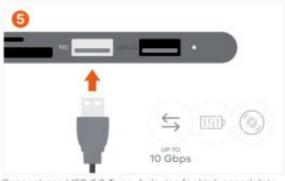
Connect one USB 3.0 Type-A device for high speed data transfer up to 10 Gbps.
