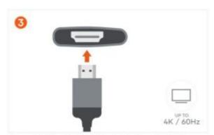
Connect HDMI cable from the adapter to a 4K HDMIequipped display. Up to 4K at 60Hz. Only supports direct HDMI connections.
