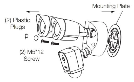
• STEP 2: Drill (2) holes on the wall and insert expansion screws. Attach gasket and fix mounting plate with screws.
