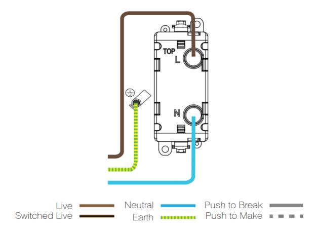
After making the connections, screw the switch plate accessory gently to the back box ensuring no wires become trapped.
