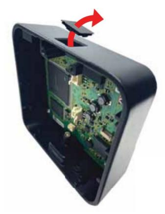
8. Slide the biometric sensor into the keypad housing ensuring the biometric ribbon is moving towards the right and over the green ground cable.
