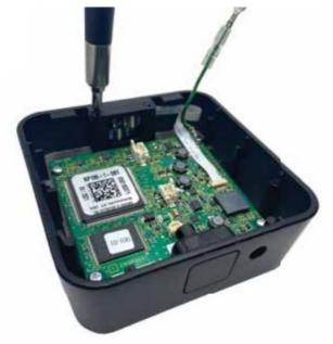
10. Slide the ribbon cable into the biometric connection.
