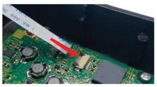
11. Push the ribbon cable connection lock down to secure the ribbon cable.
