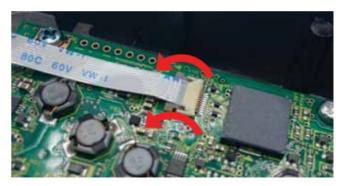
12. Check the ribbon cable to make sure the mounting of the keypad will not damage the cable.
