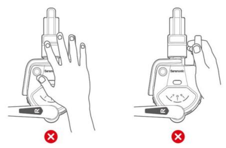
4. While using, please do not cover the antenna area shown in the figure above to avoid signal interference, and do not handle the antenna to avoid damage.
