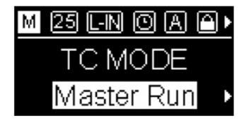
Based on your needs, you can rotate or press the knob to select the TC Mode, including Master Run, Auto Jam, and Jam Once and Lock.
