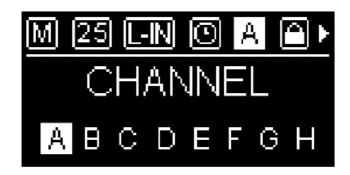
TC-NEO supports channel management, allowing devices to be assigned to channels A-H. Once TC-NEO devices are set to the same channel, timecode synchronization within the channel can be achieved through wireless synchronization technology. The default channel is Channel A. If TC-NEO needs to synchronize timecode with other Saramonic devices that support timecode, the other devices must also be set to the same channel or group to enable synchronization. Channels and groups have the same meaning.
