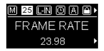
Enter this menu option to set the frame rate for TC-NEO as 23.98, 24, 25, 29.97, 29.97DF, 30, 50, and 60, making it suitable for various regions and shooting requirements. Users can select the appropriate frame rate to ensure stable synchronization and maintain consistency between video and audio.
