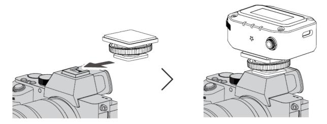
2. Install the TC-NEO or other accessories onto a tripod, bracket, or camera's cold shoe mount using the included thumb screw 1/4"-20 thread cold shoe.
