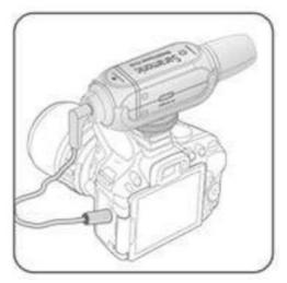
(3) Plug the supplied 3.5mm TRS to TRS output cable into the OUTPUT jack of RX-35 and then into camera's mic input.
