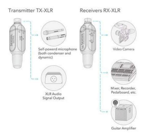
1. Attach the Blink800 TX-XLR transmitter to dynamic microphone, self-powered microphone, or other XLR audio output device.
