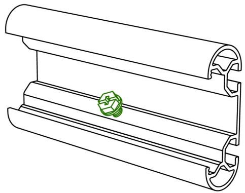
13. Mount the zone clock pole and attached housings to the bases by hanging the upper edge of the pole on the upper hooks of the base. Then, using the flathead screwdriver, turn the inner screw counterclockwise to activate the lower locking mechanism.
