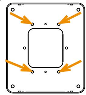
4. Remove the template and insert the wall anchors into the outer holes.
