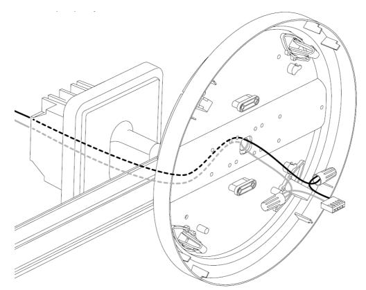
If your clock uses Power over Ethernet, use a crimp tool to insert the CAT5/CAT6 wires into the RJ45 connector.
