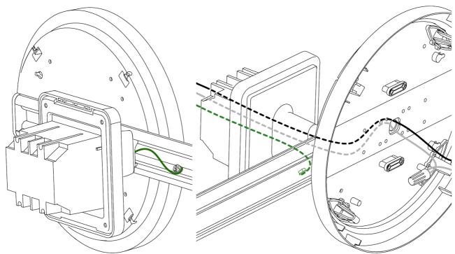
16. Run wiring or IP cables to the remaining clocks. Thread wiring through the white cable anchors where applicable (this may have already been done for you, if it is a wire-powered system).
