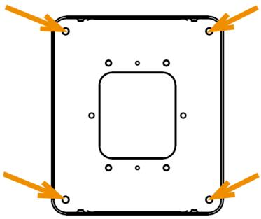
3. Skip this step if your clock is battery-powered. Use a pencil to poke through the template and find the position of each inner hole. Mark each position on the wall.
