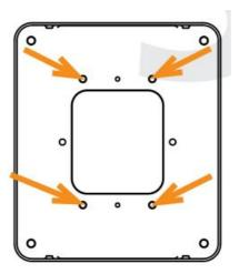
4) Remove the template and insert the wall anchors into the outer holes.
