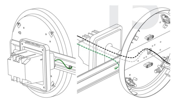
16) Run wiring or IP cables to the remaining clocks. Thread wiring through the white cable anchors where applicable (this may have already been done for you, if it is a wire-powered system). Details on how to power each clock and attach it to the housing can be found in the double-mount portion of the clock manual for your synchronization system.
