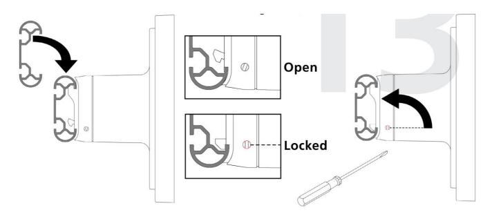
Test the pole to confirm that the locking mechanism has fully engaged. The pole should be able to slide side to side while attached to the base, but a user should not be able to lift the pole off of the base. **FAILURE TO FULLY ENGAGE THE LOCKING MECHANISM MAY RESULT IN INJURY.**
