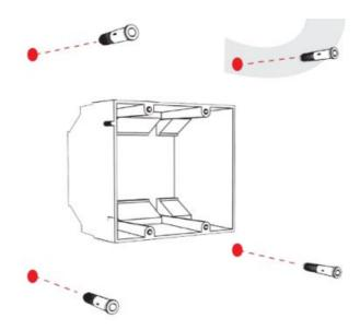
6) Insert the machine screws through the mounting plates and into the gang boxes, then insert the self-tapping screws through the mounting plates and into the wall anchors.
