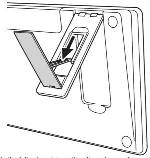
(3) Put the keyboard as shown in the following picture, then it can be used as a stand.
