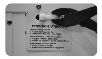
• The Santa Fe Ultra98/120 uses a compressor to power the refrigeration system. To protect the compressor and refrigeration system during shipping, a plastic tie wrap secures it to the unit's frame. Remove the tie wrap by cutting the tie wrap and pulling from the unit as shown. After removing tie wrap, insert plastic plugs provided into the holes.
