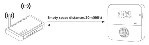
The distance varies with the environment. /A If the Receiver is too far from the router, it will not be able to connect to the smartphone.
