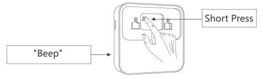
2. Short press the SOS Button, and the Receiver will stop "beep' after successful pairing.
