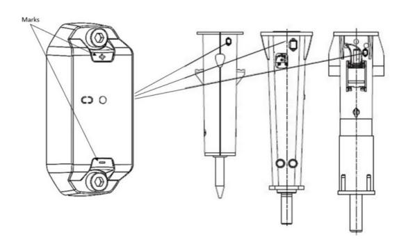
Warning! The hammer must be secured from falling down in any direction when handling it.
