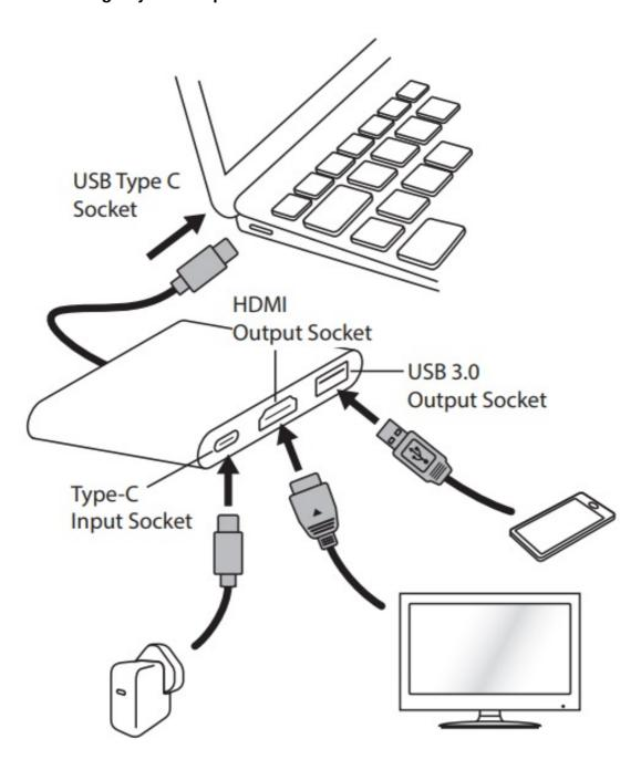
Type-C input socket for power input only.
