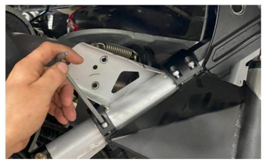
10. Insert the 5/8" x 3" bolt and washer through the bump stop housing and trunk support bracket with threads inbound. You will only have a few threads showing on the inbound side.
