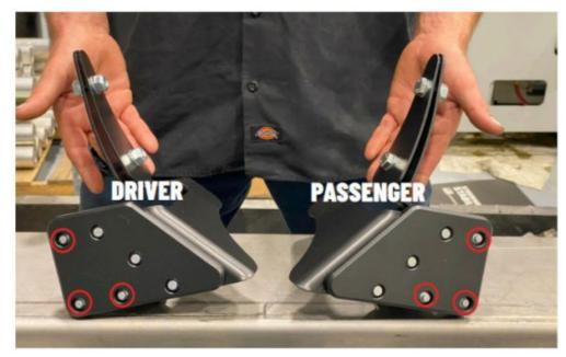
2. Sandwich the bump pad brackets on either side of the trailing arm and loosely install all hardware. The brackets install over the brake line. You will torque these bolts later.
