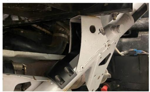
7. Raise and slide the passenger side bump stop up under the frame and trunk support pocket inserting the fork into the factory tie down knob.
