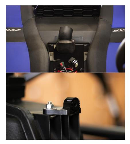
Install the L Brackets (F) onto the Adapters with the Screws (K) and Washers (I), selecting the proper angle and orientation based on the desired location for the Particle Separator. Apply Thread Locker to the screws before installing, then tighten.
