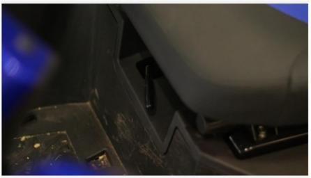
Remove the center console cover by lifting up on the back and sliding the front tab out from its slot. Make sure the rear mounting grommets did not pull out with the cover.
