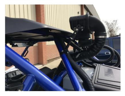
Once you are satisfied with the position of the Particle Separator, tighten the Straps, double check that all mounting screws and nuts are tight and that they are securely mounting the Particle Separator on the roll cage.
