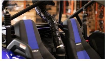
Secure the Flex Duct to the roll cage with Velcro.
