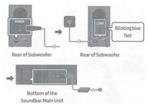
The LINK LED indicator stops blinking and glows a solid blue when a connection is established between the Soundbar and the Wireless Subwoofer.
