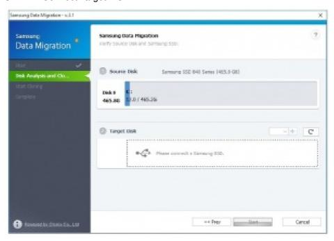
3. If the Target Disk is connected, the status of the Target Disk is displayed on the screen. \* You may need a separate M.2 PCIe/USB converter (connector) to connect an NVMe SSD.
