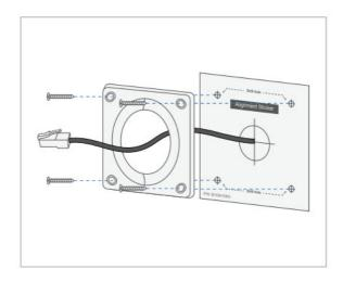
If necessary, install drywall anchors using the alignment sticker for reference. Feed the ethernet cable through the middle opening of theback plate, then fasten the backplate to the mounting surface using the provided screws.
