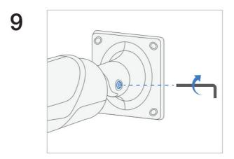
Tighten the camera pan screw with the Torx driver.
