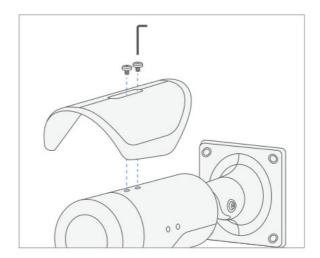
If using the SC21 in an outdoor deployment, attach the sunshield using the provided screws and Torx Driver provided.
