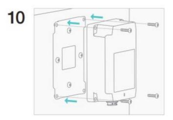
Mount AG onto mounting plate with 4 flat-end screws (bag 2).
