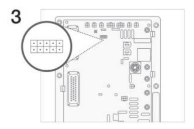
For models prior to 2017 without a BlueBox, connect the REB iBox to the J98 10-pin connector on the control board.
