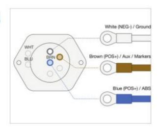
Connect the cable to 7-way. AG light turns on for 30 seconds if correct.
