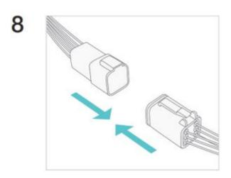
Connect Samsara cable to iBox/BlueBox harness via the 6 pins Deutsch connector.
