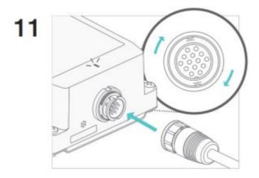
Plug cable into AG, twist to lock. The LED light will blink orange while connecting and turn to a solid green light once connected. If the light turns solid orange, ensure you're in an area with a good cellular signal. For further troubleshooting tips, refer to your asset gateway troubleshooting guide.
