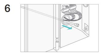
Open Thermo King cabinet and electronics control box (may require unbolting). Route reefer end of Y-cable into control box via rear grommet.
