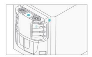
Determine the desired location of AG24: place as high on the trailer as possible in order to maximize GPS signal, but avoid protruding unit above the trailer roofline to avoid potential damage.
