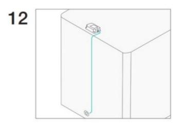
Run the cable to 7-way. Fasten to the trailer with zip ties.
