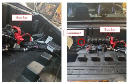
Step 3: Instal I Cont rol ler, Relay, and Fuse
