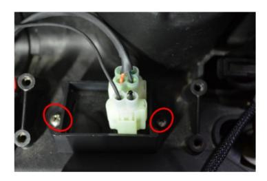
Step 2: Plug-In and Secure Backup Beeper, and attach leads
