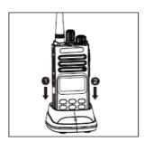
As 8 shown, connect the power adapter to AC power socket and the jack at the back of the charger.
