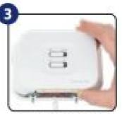
Remount the front housing. Tighten the screws located on the bottom of the housing receiver.
