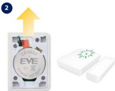
After removing the plastic battery tab, the LED will flash green intermittently
