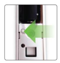
Keep the reset button pressed for 4 seconds when inserting back the battery. The device will reset and enter pairing mode.
