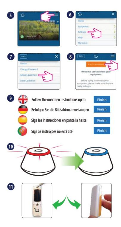
Install the slim window/door senor using the screws or the double-sided tape.
