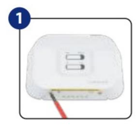
• Mount the back housing of the receiver, and then connect wires according to the appropriate schematic for your heating device.
