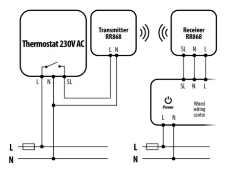
Solution when there is no enough wires between thermostat and a wired wiring centre
