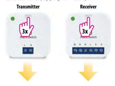
3. LED diodes will flash orange on both devices.
