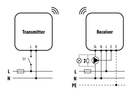
When S1 transmitter contact is closed, receiver sends 230V AC (SL output).
